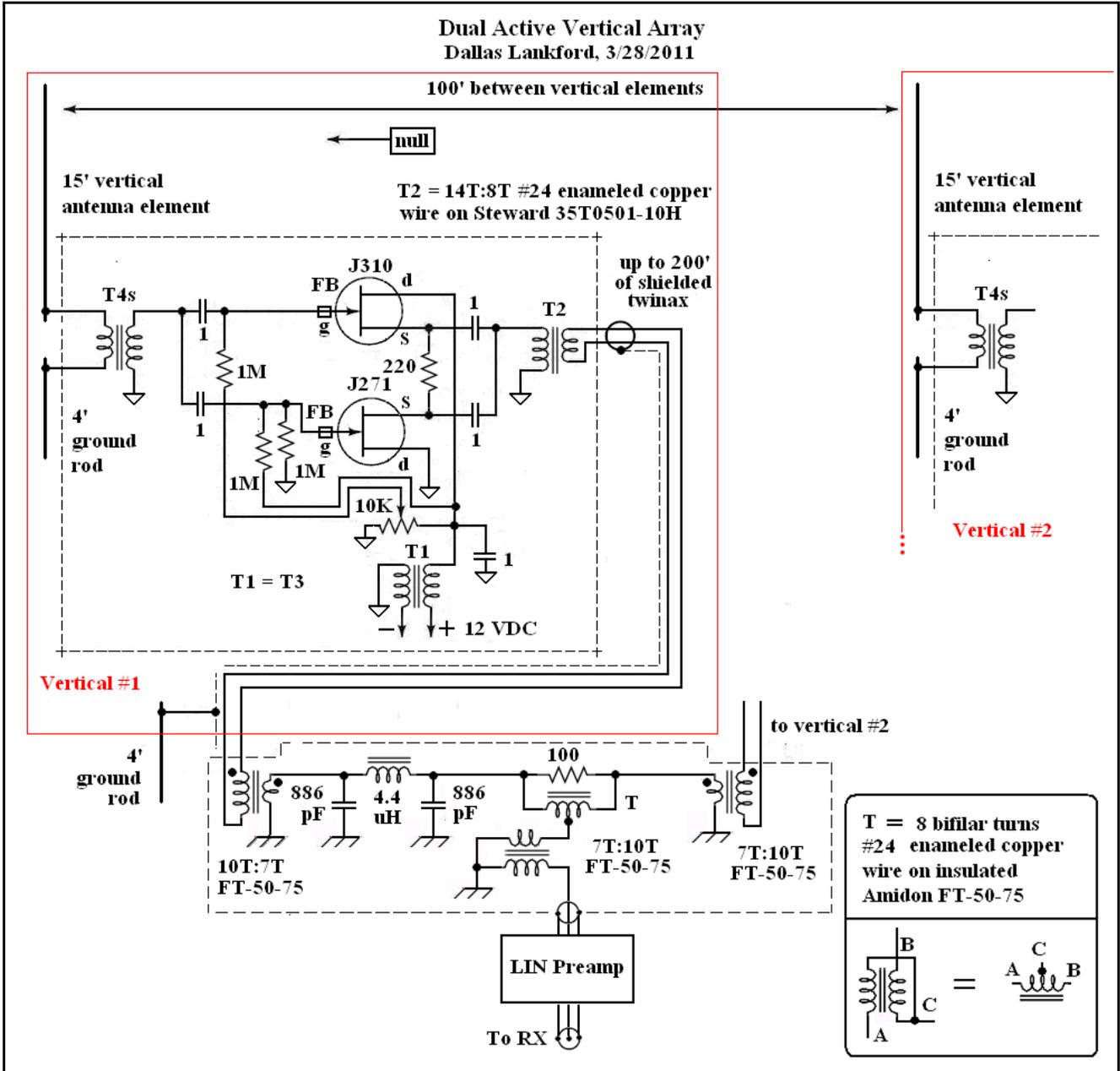
The actual test setup used two 13.6 dB gain LIN preamps at the phaser ends of the 200' lengths of shielded twinax, each PPL connected to the phaser by a short length of coax.
