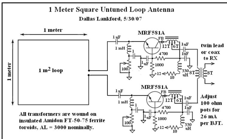
Originally a 6 turn to 3 turn step down transformer was used at the input of the amplifier which was consistent with the posting recommendation. Later, after measurements of loop inductance, amp input resistance, and amp gain, the input transformer was deleted; more details of this change are found near the end of this article.
